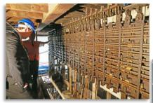
Above - We often get asked about the locking mechanism. Here Steve Growcott is explaining to Matt Walsh how the device works to safeguard the signalling of trains.
